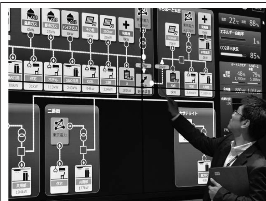
Photo: Yoshikazu Tsuno/AFP/Getty Images Multiple Input, Multiple Output: The Kashiwanoha smart-city project uses energy from electric-vehicle batteries, biogas, storage batteries, solar panels, and the grid.
